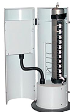
Figure 2. NanoMoudi particle size-selected collector.
